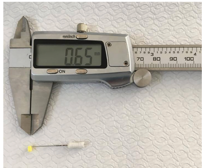
Figure 2. Digital caliper with 0.01 mm precision and endodontic spreader of 10-gauge.
