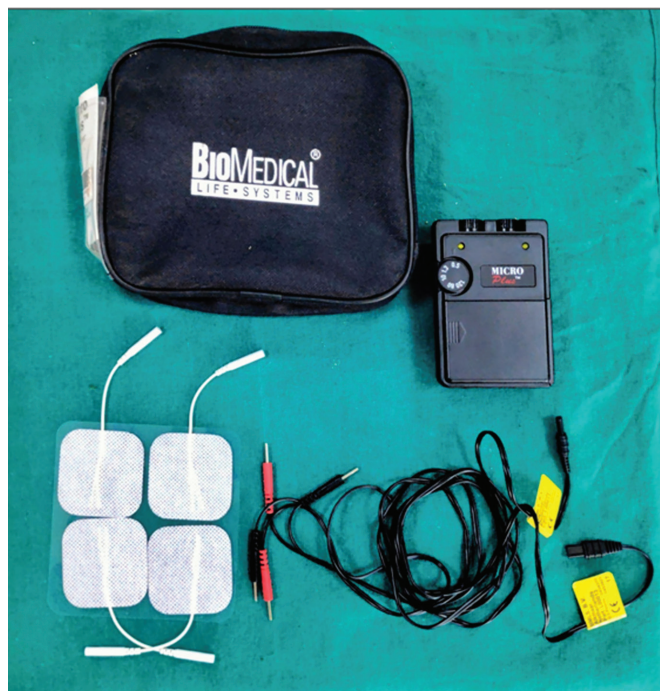
Figure 1. Transcutaneous electrical nerve stimulation machine with surface electrodes
