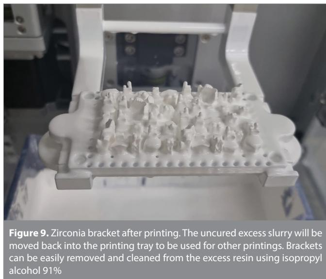
**Figure 9.** Zirconia bracket after printing. The uncured excess slurry will be moved back into the printing tray to be used for other printings. Brackets can be easily removed and cleaned from the excess resin using isopropyl alcohol 91%
