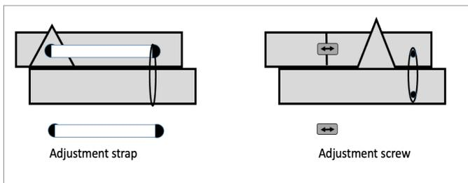
**Figure 1.** The illustration of the traction type of MAD (left) and the fin coupling type of MAD (right). The traction type of the appliance is adjusted by different lengths of the straps. The fin coupling type of device is adjusted using a screw in the upper jaw, which pushes the lower jaw forward with the help of a wing.
